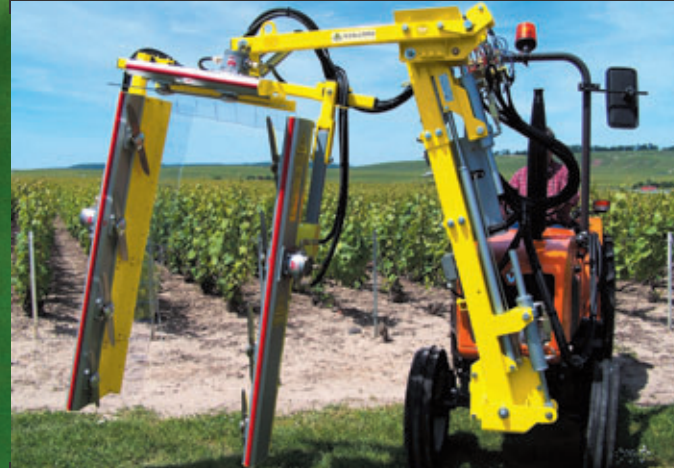
P3000 LZF Multi purpose Reinforced frame, 1 SE + 5 DE. Equipped with a fast fixing. This frame allows the fitting of the leaf remover.
