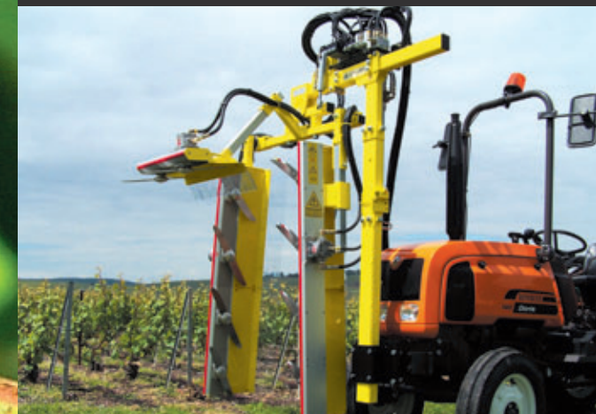
P3000 LP 1 complete row for a front or side mounting 3 cylinders: 1 UP/DOWN – 1 IN/OUT – 1 UPPER SLOPE.
