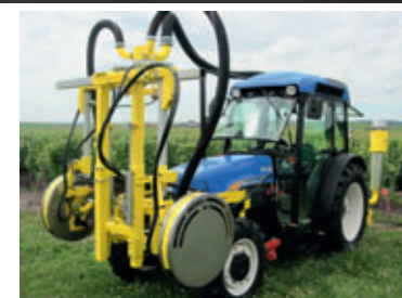
Leaf remover on inter-row tractors.
