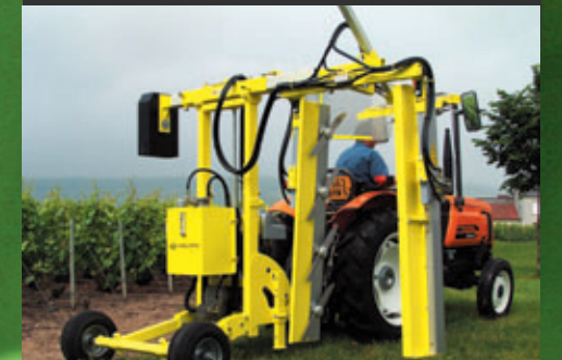
REAR MACHINES ON P.T.O. 2 complete rows – 2 half rows or 1 complete row.
