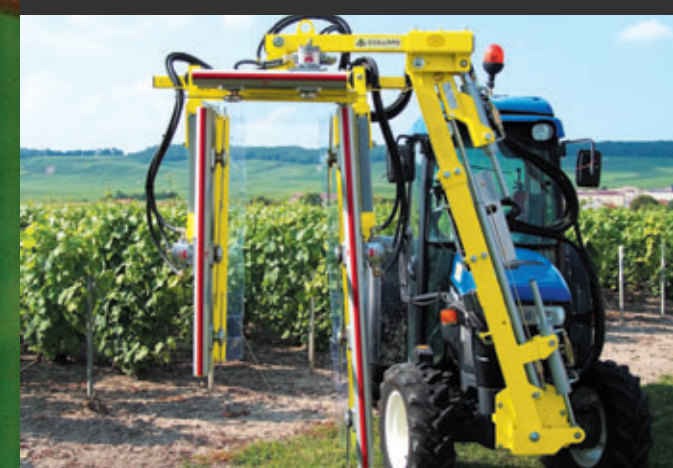
P3000 LZF Standard equipped with an oscillating frame with hydraulic parallelogram.
