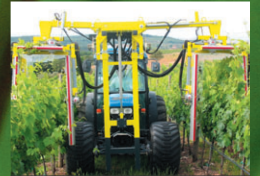
P3200 I 2 complete rows front mounted with up to 7 cylinders.
