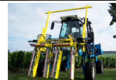
Vine trimmer on straddle tractors.
