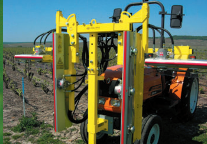
P2200 MIDI 2 half rows at the front. Special for narrow spacing. 1 UP/DOWN. Equipped with a single tube frame.
